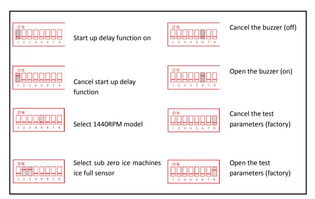
Eight-bit DIP switches on the centre of the PC board (Figure 3-1) are from left to right. Override is when dip switch is in the on position.
