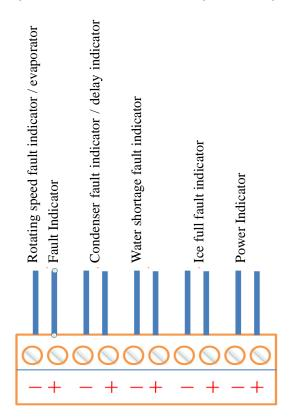
b) Ice machine external indicator (small board) wiring diagram
