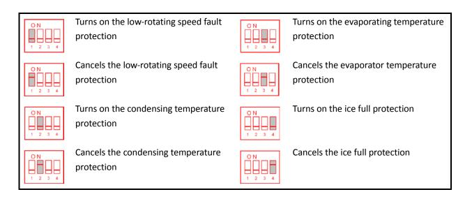
Four-bit DIP switches on the center of the PC board (Figure 3-2) are in order from left to right.
