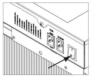
6. To clean/sanitize ice transport tube – Press power switch OFF
