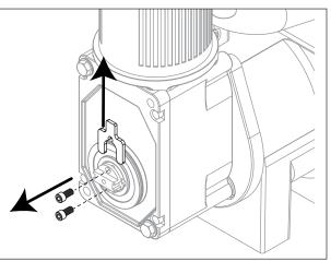
3. Remove gearbox insulation.
