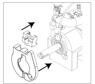
23. Install shuttle drain tube and front feed water tube (Fig. 24).
