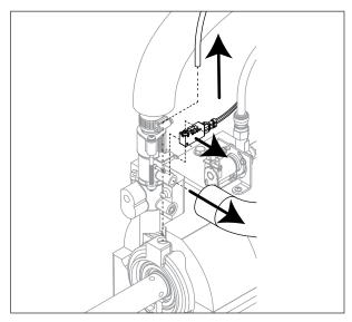
**9.** Remove front feed water tube from push-in fitting, shuttle drain tube, and shuttle switch.
