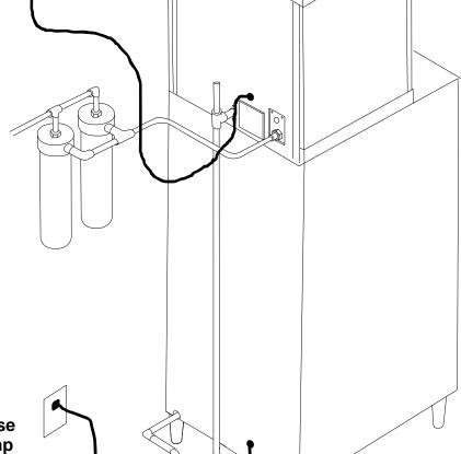
Caution: Do not use a condensate pump in place of a floor drain.
