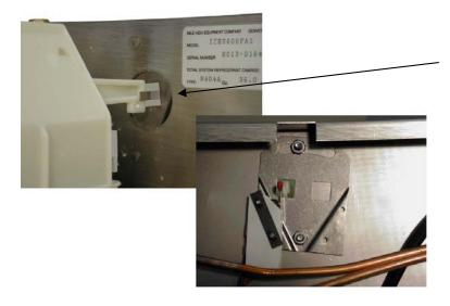
Water splash curtain actuator tab positioned behind bin switch
